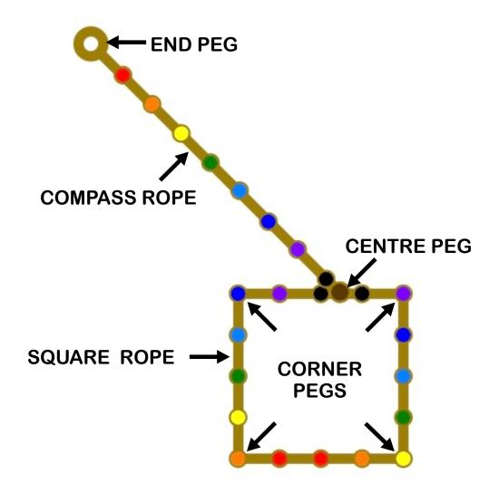
The CENTRE PEG marks the centre of your labyrinth. Position the CENTRE PEG in the centre of your chosen area, then extend the COMPASS ROPE in all directions, to check that you have enough flat, open ground for your labyrinth.
